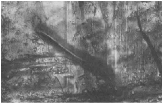
Fig. 18. SEM photograph of extrudate of blend (B') at 500\times .
